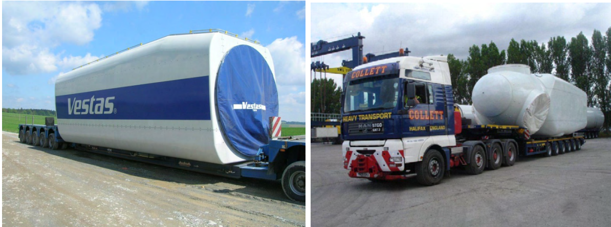
Figure 2-6: Transportation of a Nacelle
